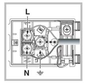
1. Open the terminal board by inserting a screwdriver into the side tabs of the cover. Use the screwdriver as a lever by pushing it down to open the cover (see diagram). 2. Install the power supply cable by loosening the cable clamp screw and the three wire contact screws L-N-Connect the wires to the corresponding terminals: the Blue wire to the terminal marked (N), the Brown wire to the terminal marked (L) and the Yellow/Green wire to the terminal
